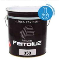
2-component solvent-free sanitary epoxy paint. High resistance to solvents, mineral oils and chemicals in general. Can be applied in thicknesses of up to 250 micro humidity. Its use as a coating for drinking and waste water containers and food products in general is particularly noteworthy.
